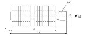
Coaxial fixed terminations absorb RF& microwave energy and are commonly used as dummy loads of antenna and transmitter. They are also used as match ports in many multiport microwave device such as circulator and directional coupler to make these ports which are not involved in the measurement be terminated in their characteristic impedance in order to ensure an accurate measurement.
