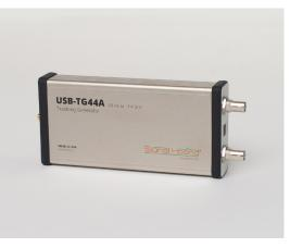
The Signal Hound TG44A is a USB-powered, 10 Hz to 4.4 GHz, economy tracking generator and CW signal generator. The TG44A turns your SA44B, SA124B, or BB60C spectrum analyzer into a versatile scaler network analyzer. The combination can measure gain, frequency response, compression, flatness, and insertion loss on components and subsystems.
