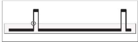
Fig. 3-5 No triggering due to AC coupling of signal with low duty cycle.
