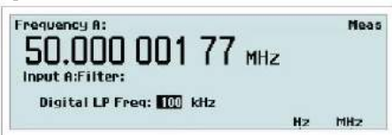
Fig. 3-7 Value input menu for setting the cutoff frequency of the digital filter.
