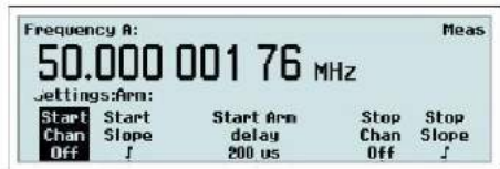
Fig. 2-14 CNT-90 & CNT-90XL: Setting arming conditions.
