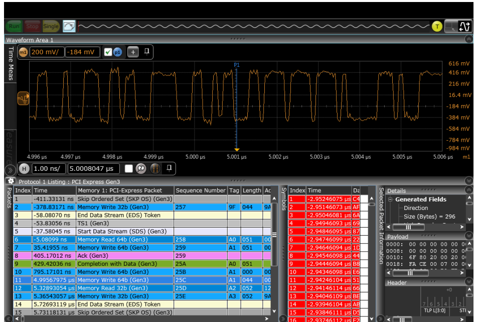
Z-Series decoding the PCI Express Gen 3 packets.
