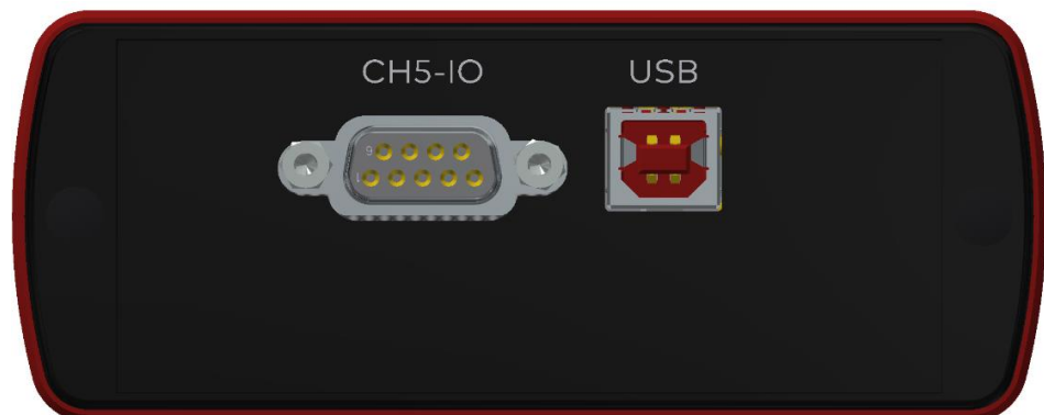
Figure 40: VN1640A with D-SUB9 connector and USB
