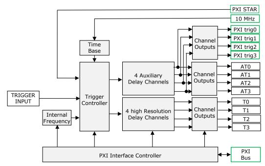
Note: Signals with green border are connected to PXI bus
