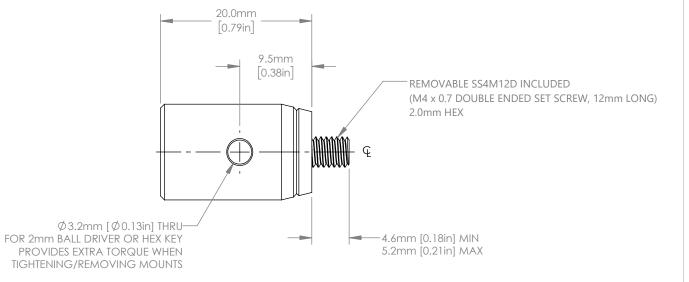
DRAWING PROJECTION  $\bigoplus$ www.thorlabs.com NAME DATE 20mm LONG METRIC TR-SERIES POST 28/MAR/13 AVREDRAWN MATERIAL 04/APR/03 AC **APPROVAL** STAINLESS STEEL COPYRIGHT © 2013 BY THORLABS APPROX WEIGHT ITEM # VALUES IN PARENTHESIS ARE CALCULATED AND MAY CONTAIN ROUNDOFF ERRORS
