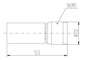
Coaxial fixed terminations absorb RF& microwave energy and are commonly used as dummy loads of antenna and transmitter. They are also used as match ports in many multiport microwave device such as circulator and directional coupler to make these ports which are not involved in the measurement be terminated in their characteristic impedance in order to ensure an accurate measurement.
