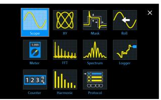
$\ensuremath{\mathbf{8}}$  instruments in one – select the instrument you need at the push of a button.
