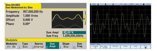
Dual-tone signal created by summing waveforms using the modulation type "Sum".
