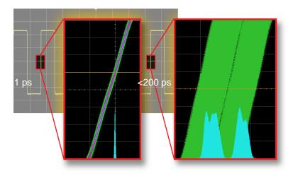
True*form* technology shown on the left significantly improves jitter performance compared to a traditional function generator shown on the right.
