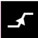
The EasyRamp function configures a constant rise of supply voltage within a set time frame. The output voltage can be increased continuously within a 10 ms to 10 s with 1 ms step size. Each channel has an independent ramp configuration. See [Figure 6-23](#).
