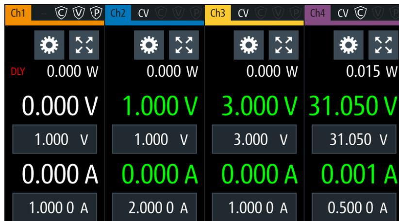
Figure 6-7: Delay text at channel display area
