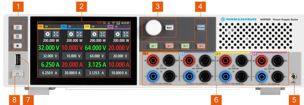
**Figure 4-2: Front panel of R&S NGP800 power supply**
