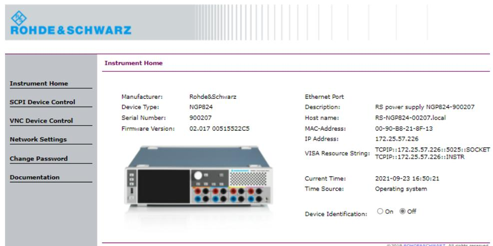
Figure 6-50: Instrument home webpage of a power supply model
