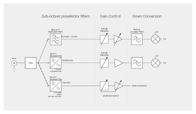
The SM200A/B is essentially a low IF receiver. We chose this architecture to complement our low phase noise local oscillator (LO), while avoiding the shortfalls of zero IF (direct) conversion, and because of the availability of high linearity direct conversion demodulators and I/Q mixers.
