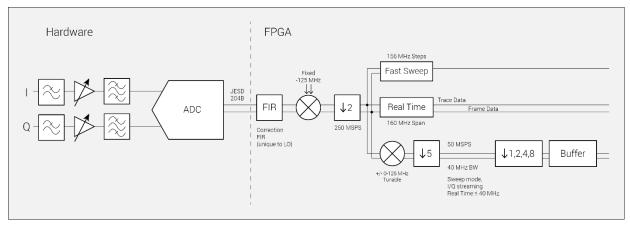
The digitized data is processed with a special FIR filter to reject the image response and flatten the frequency response. This data is then digitally tuned to select the lower sideband, decimated down to 250 MSPS I/Q, and distributed to several signal processing blocks within the FPGA.
