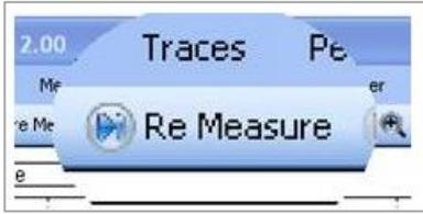
In a re-measurement, a second measurement is performed for each frequency with an entry in the peak list. This measurement is performed with a special standardized evaluation process (quasi peak). The re-measurement is always performed with the quasi peak detector and cannot be adjusted. The results of this measurement are relevant for the adherence to the EMC standards.
