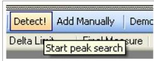
For instance, if the increment is 60kHz and the width is set to 10 points, the increment equals  $10 \times 60\text{kHz} = \pm 600\text{kHz}$ . Consequently, the peak value detection is performed in 600kHz increments (to the left and right of the peak).
