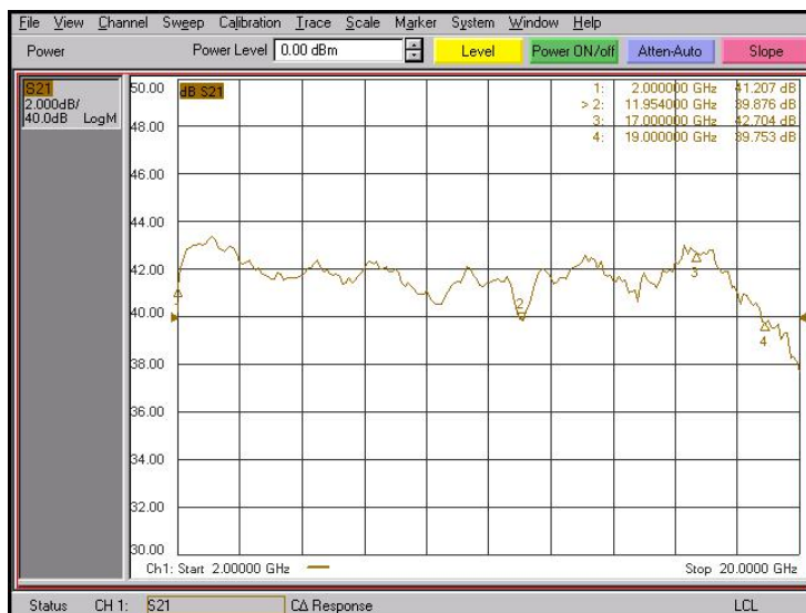
Graph2: Power Gain @ Pin=0 dBm (Ambient temp. +25±3°C, LOAD VSWR ≤ 1.3)
