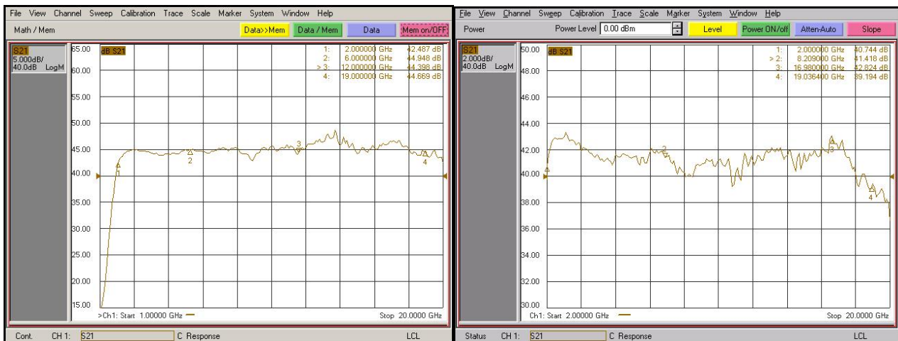
Figure left: Power Gain@ Pin=0 dBm (Ambient temp. -40±3°C)
