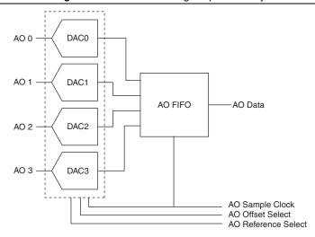
Figure 5-1. M Series Analog Output Circuitry
