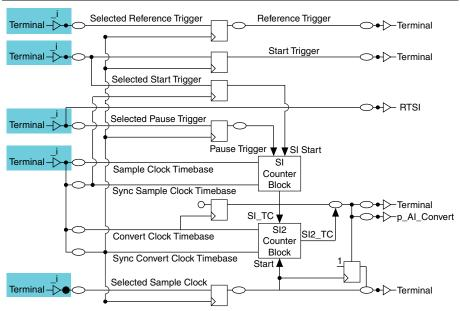
Figure B-3. Input Timing Diagram
