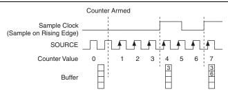
Figure 7-4. Buffered (Sample Clock) Edge Counting
