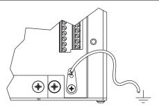
(USB-62xx BNC Devices) You can attach a wire to a CHS GND screw terminal of any USB-62xx BNC device, as shown in Figure 1-5. Use as short a wire as possible. In addition, the wires in the shielded cable that extend beyond the shield should be as short as possible.
