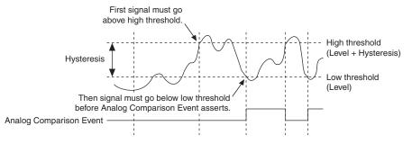
Analog Window Triggering—An analog window trigger occurs when an analog signal either passes into (enters) or passes out of (leaves) a window defined by two voltage levels. Specify the levels by setting the window Top value and the window Bottom value.
