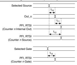
Table B-34. Output Delays Timing
