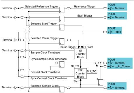
Figure B-20. Output Timing and the Analog Input Timing Engine
