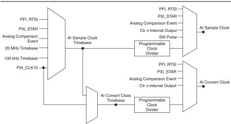
Figure 4-12. Analog Input Timing Options
