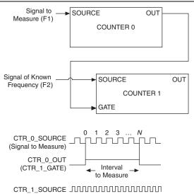
Then, route the Counter 0 Internal Output signal to the Gate input of Counter 1. You can route a signal of known frequency (F2) to the Counter 1 Source input. F2 can be 80MHzTimebase. For signals that might be slower than 0.02 Hz, use a slower known timebase. Configure Counter 1 to perform a single pulse-width measurement. Suppose the result is that the pulse width is J periods of the F2 clock.
