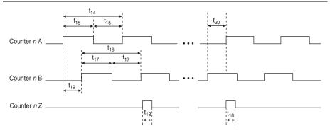
Table B-35. Quadrature and Two Pulse Encoder Timing
