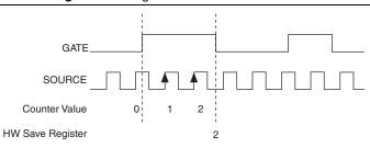
Figure 7-5. Single Pulse-Width Measurement
