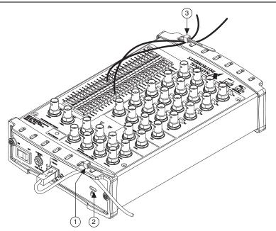
Figure 1-7. USB Cable Strain Relief on USB-62xx BNC Devices
