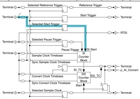
Figure B-12. Sample Clock Timebase Timing Diagram
