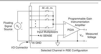
Note (NI USB-62xx BNC Devices) To measure a floating signal source on USB BNC devices, move the switch under the BNC connector to the FS position.
