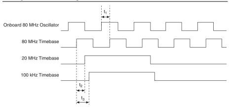
Table B-36. Generating Different Clocks from the Onboard 80 MHz Oscillator
