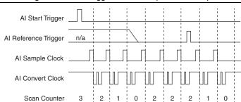
Figure 4-15. Pretriggered Data Acquisition Example
