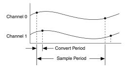
AI Convert Clock controls the Convert Period, which is determined by the following equation:
