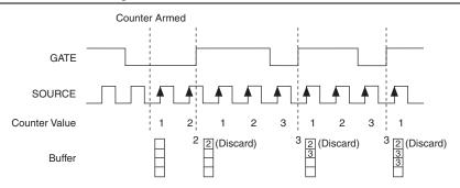
Note that if you are using an external signal as the Source, at least one Source pulse should occur between each active edge of the Gate signal. This condition ensures that correct values are returned by the counter. If this condition is not met, consider using duplicate count prevention, described in the *Duplicate Count Prevention* section.
