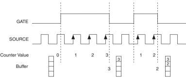
Note that if you are using an external signal as the Source, at least one Source pulse should occur between each active edge of the Gate signal. This condition ensures that correct values are returned by the counter. If this condition is not met, consider using duplicate count prevention, described in the *Duplicate Count Prevention* section.
