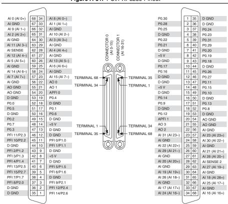
Figure A-31. PCI/PXI-6289 Pinout
