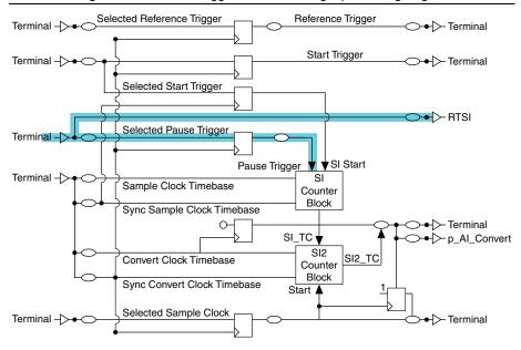
Figure B-19. Pause Trigger Timing Diagram
