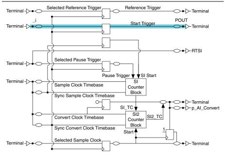
Figure B-10. Convert Clock Timebase Timing Diagram
