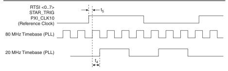
Table B-37. Generating Different Clocks Using an External Reference Clock and the PLL
