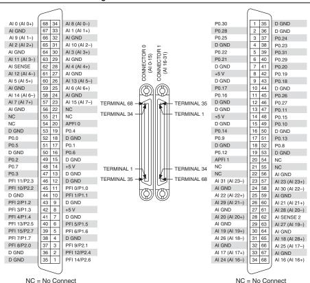
Figure A-30. PCI/PXI-6284 Pinout
