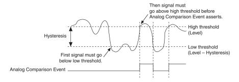
Analog Edge Trigger with Hysteresis (Falling Slope)—When using hysteresis with a falling slope, you specify a trigger level and amount of hysteresis. The low threshold is the trigger level; the high threshold is the trigger level plus the hysteresis.
