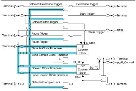
Figure B-5. Al Timing Clocks Timing Diagram
