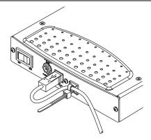
(USB-622x/625x BNC Devices) Thread a zip tie through two of the strain relief holes on the end cap to provide strain relief for your USB cable as shown in Figure 1-7. The strain relief holes can also be used as cable management for signal wires to/from the screw terminals and BNC connectors
