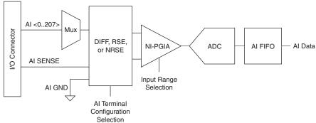
The main blocks featured in the M Series analog input circuitry are as follows:
