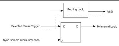
Figure B-34. Pause Trigger Output Routing Delay Timing Diagram
