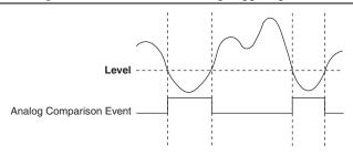
In above-level analog triggering mode, shown in Figure 11-4, the trigger is generated when the signal value is greater than Level.
