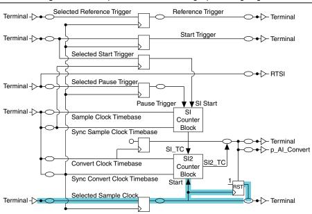
Figure B-15. Sample Clock and the Analog Input Timing Engine
