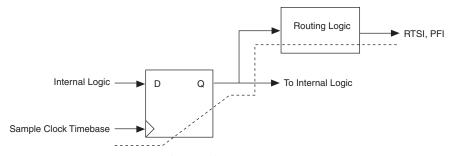
Figure B-36. Sample Clock Delay Timing Diagram
