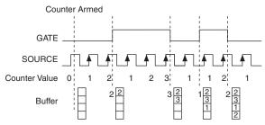
Note that if you are using an external signal as the Source, at least one Source pulse should occur between each active edge of the Gate signal. This condition ensures that correct values are returned by the counter. If this condition is not met, consider using duplicate count prevention, described in the *Duplicate Count Prevention* section.
