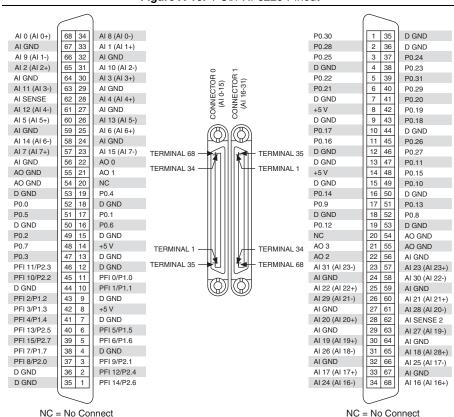
Figure A-10. PCI/PXI-6229 Pinout
