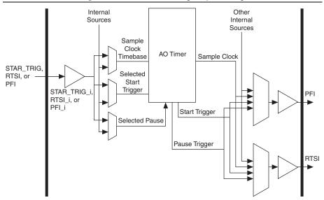
Figure B-22. M Series Analog Output Timing
