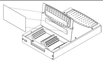
Figure 1-2. Applying the USB-62xx Screw Terminal Signal Label
