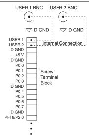
Figure 3-2 shows an example of how to use the USER 1 and USER 2 BNCs. To access the PFI 8 signal from a BNC, connect USER 1 on the screw terminal block to PFI 8 with a wire.
