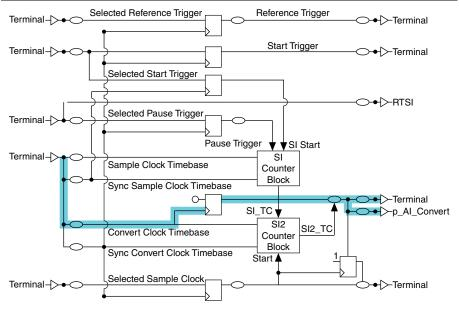
Figure B-7. Convert Clock Timing Diagram
