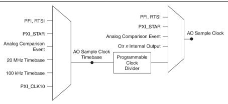
M Series devices feature the following AO (waveform generation) timing signals:
