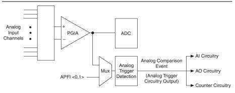
You must specify a source and an analog trigger type. The source can be either an APFI <0,1> terminal or an analog input channel.
