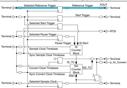
Figure B-13. Reference Trigger and the Analog Input Timing Engine
