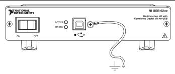
(USB-6225/625x/628x Screw Terminal Devices) You can attach and solder a wire to the chassis ground lug of certain USB-62xx Screw Terminal devices, as shown in Figure 1-4. The wire should be as short as possible.
