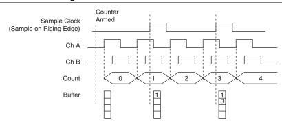
Figure 7-19. Buffered Position Measurement
