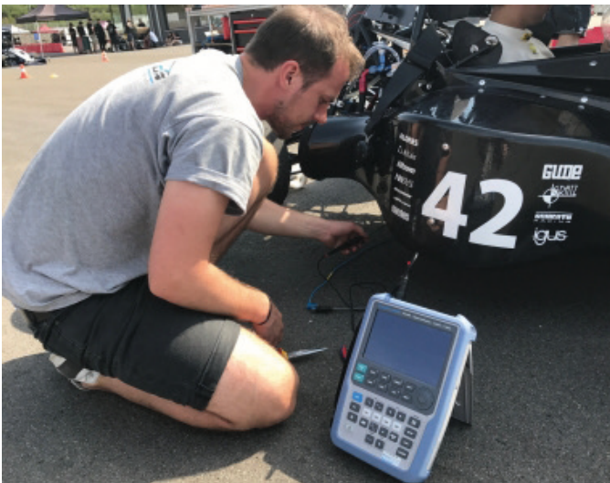
Niklas Waldstein measuring the engine control unit of the F17 to test ignition interruption
