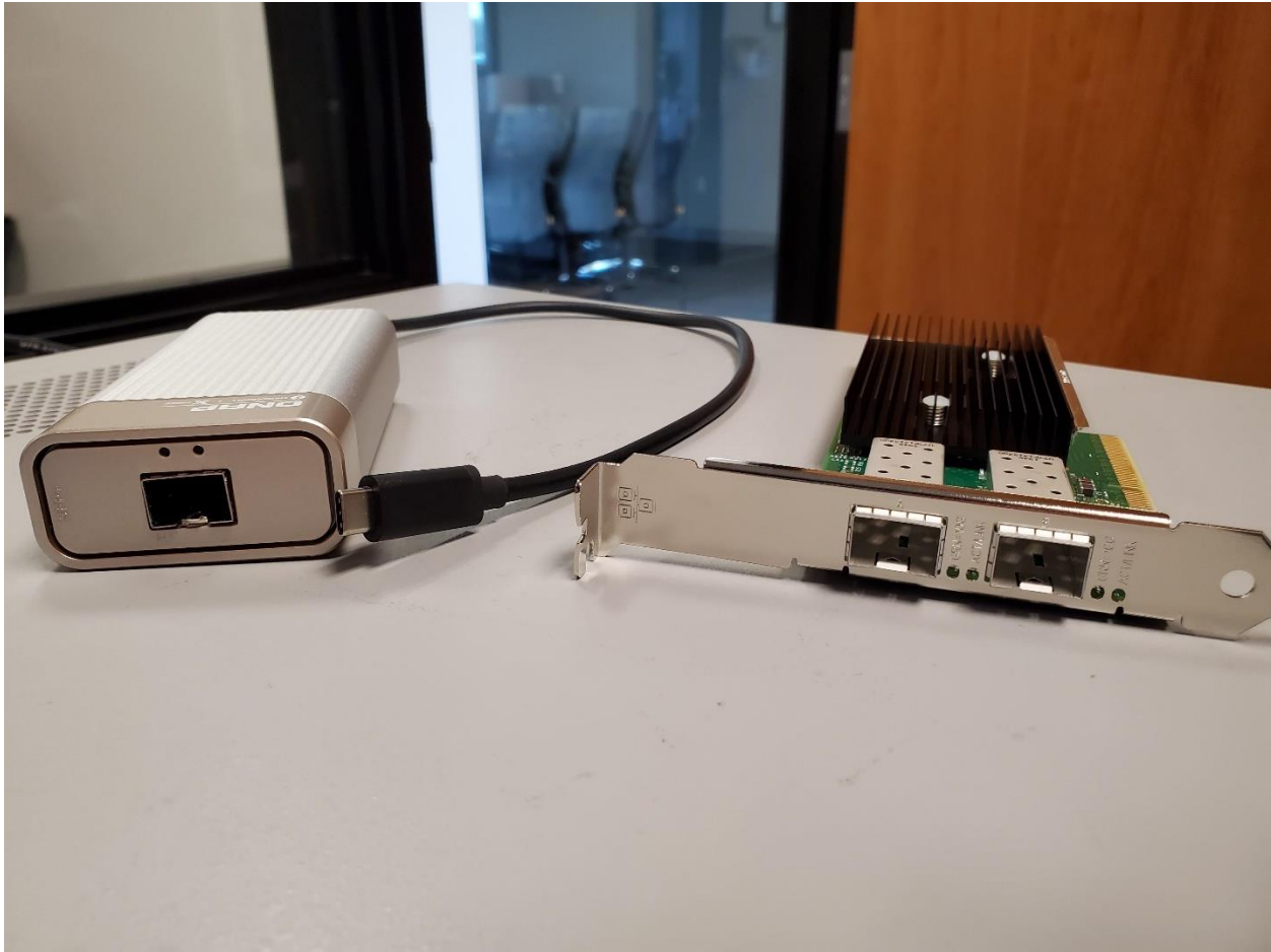
Figure 5: Left to right, Thunderbolt 3 to SFP+ adapter and 2xSFP+ 10GbE NIC adapter card.
