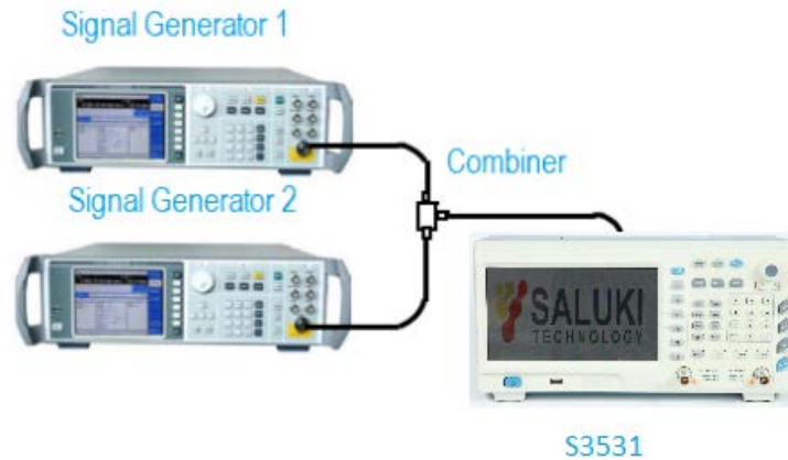
Fig 5-2: Equipment Connection for 2 signal capture
