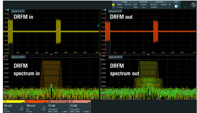
R&S®RTP multichannel frequency analysis of DRFM input and output
