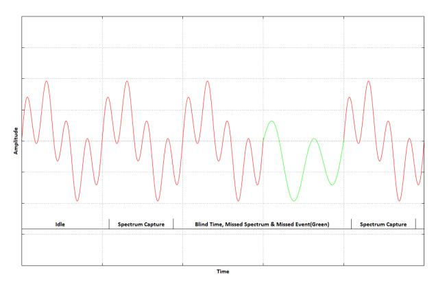
In this image we see an event missed due to the blind time between spectrum sampling. With Real-Time spectrum analysis we can prevent this and capture ALL possible events.
