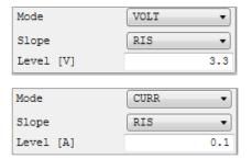
A threshold (function "Level") can also be set, as well as the offset between the rising (RIS) and falling edges (FALL) via drop-down menu "Slope".
