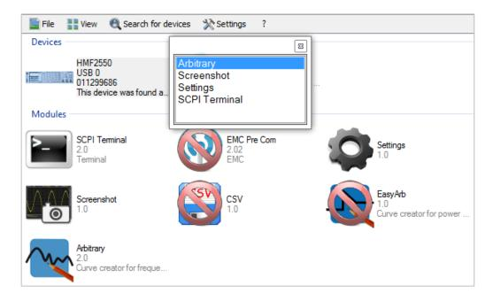
Double clicking the already integrated instrument opens a dialog box which shows the supported software modules. Double click the desired software module to start the module. It is also possible to start the software module via ENTER button if the module has previously marked by using the mouse (highlighted in blue).
