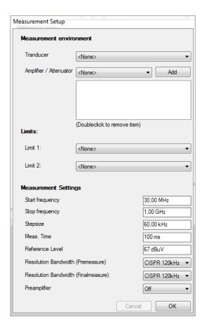
Use the Setup window to enter the necessary measurement configurations that are required by the respective EMC standard.
