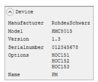
In the "Device" menu the device serial number, the installed options and the device firmware are displayed.
