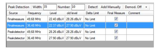
You can use right click → "Remove marker" or the Marker menu to delete a selected marker value from the list. Use right click → "Remove all" or the Marker menu to remove all marker values from the marker list.. Use right click → "Add to peak list" or the Marker menu to copy the selected marker to the peak list.
