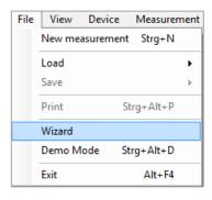
Use "File" → "Wizard" to start the internal software wizard which guides you through all required steps of the measurement setup. You can either select the settings for amplifier/attenuator, transducer and limit lines from the list or use the option "New" to enter them with the CSV Editor. The measurement settings are entered manually.
