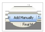
If you wish to include a frequency in the remeasurement that was not detected in the peak value detection, you can click on "Add Manually" to generate an entry in the list. In this case, the value is entered manually. The entry is shown in the peak list with the comment "Manual". Therefore, any number of locations in the spectrum can be marked and measured.
