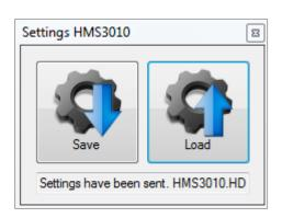
The function "Load" allows you to load instrument settings from a PC back into the measurement instrument. Click the "Load" button to open a dialog box which allows you to select the respective settings file. Click the "Open" button to transfer the instrument settings. If the instrument settings have been successfully loaded and transferred to the measurement instrument, this will be displayed in the module window.
