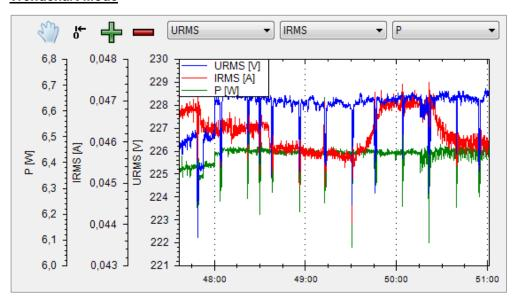
Using display mode "Trendchart" current or voltage values can be displayed as a signal profile (similar to the roll mode in an oscilloscope). Compared to the "trendchart" display mode on the instrument the "Trendchart" display mode via power analyzer software is used to show up to three selected values over time simultaneously.
