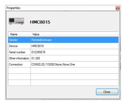
Right click the inserted device or a software module to open a "Properties" window which shows the properties of the device (e.g. device type, serial number, etc.) or of the selected software module (e.g. module type, supported devices etc.). Use "Close" to close the properties window.
