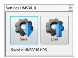
Click the "Save" button to open a dialog box which allows you to select the respective location (folder) and a file name. Click the "Save" button again to save the selected settings. If the instrument settings have been successfully saved on the PC, this will be displayed in the module window.
