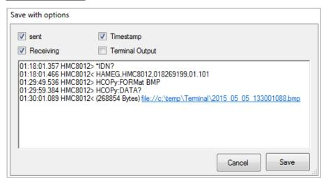
This function allows the output parameters to be filtered and saved. The following options can be activated or deactivated:
