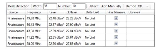
The frequency value can be adjusted for manually inserted peak values. Depending on the entry origin, the level values will be determined in different ways:
