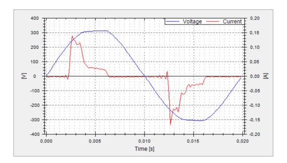
The "Waveform" display mode can be used to display the voltage (blue) and current (red) simultaneously as a trace on the screen (hardware-based triggering). Exactly one signal period is displayed in the measurement diagram and automatically scaled to the measuring range final value (100kHz max.).
