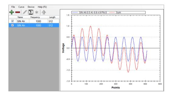
If one waveform is shorter than the other, the missing points will be filled with the value  $\mathbf{0}$ .
