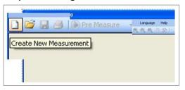
Use "Create new measurement", Wizard ("File" → "Wizard" or "File" → "New measurement" to create a new test set configuration. This opens the Setup window where you can select all necessary settings. Settings for transducer, amplifier/attenuator and limit lines are defined in advance based on the previously described procedure.
