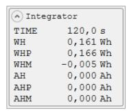
In the "Measurement" menu an energy counter can be activated. The recorded integrator values will be displayed in the middle section of the power analyzer software ("Integrator" menu). WHP / AHP represent the power / current in the positive direction and WHM / AHM in the negative direction. WH / AH correspond to the sum of the watt-hour/ ampere-hour positive and negative portions, respectively.
