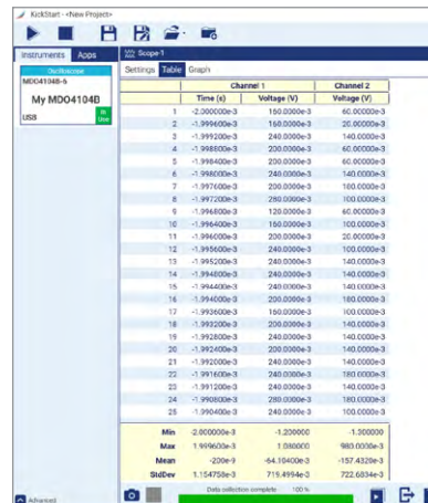
Data collected from the scope can be displayed in Table View with statistics.
