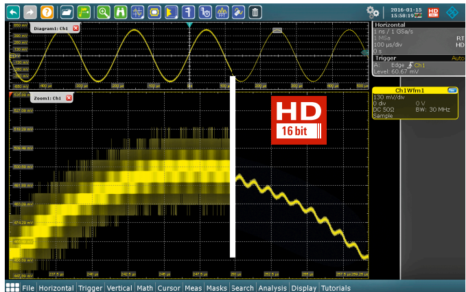
The 16-bit HD mode makes signals details visible that are otherwise hidden in noise
