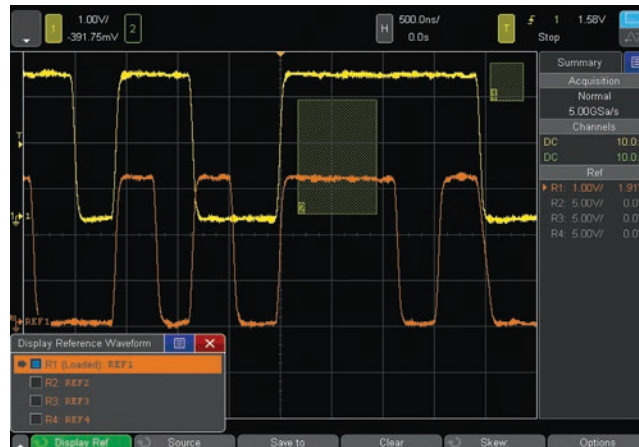
Figure 34. Store and recall up to four reference waveforms.
