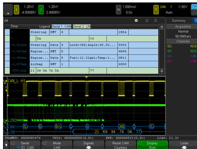
Figure 20. Dual serial bus CAN and LIN decode and interleaved "lister" display.
