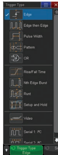
Figure 43. Wide array of advanced parametric trigger modes.
