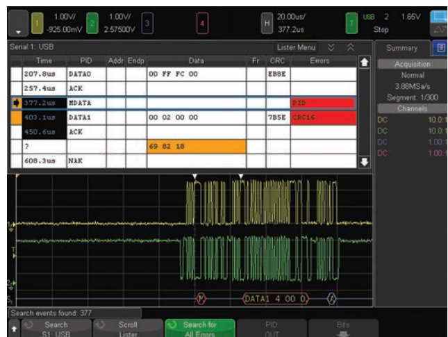
Figure 21. USB 2.0 trigger, decode and "lister" display.
