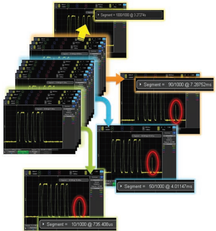
Figure 7. Segmented memory efficiently manages the memory to capture up to 1,000 segments of interest to you, making it an effective ultra-deep memory oscilloscope that can easily capture infrequent events and anomalies.
