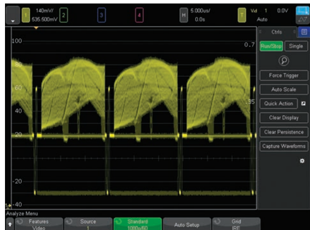
Figure 27. Triggering on 1080p HDTV signal analysis.
