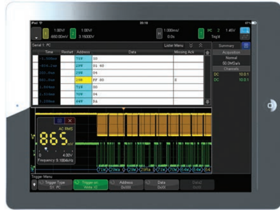
Figure 38. Tablet virtual front panel control.
