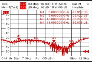
Note: Input/output return loss measurements include attenuators to protect equipment
