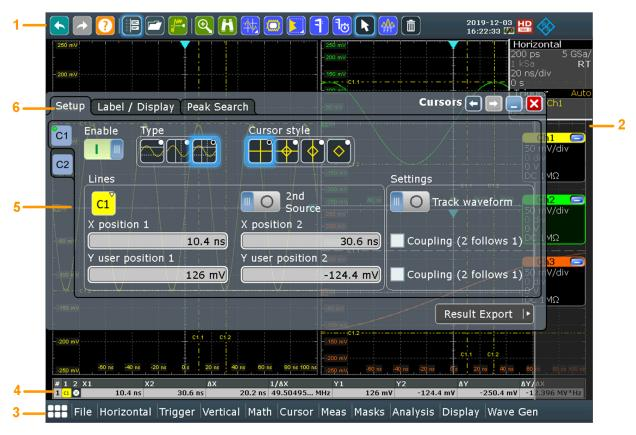
Figure 7-4: Control elements on the touchscreen
