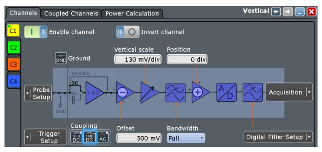
If you use a passive probe, you can filter the DC component by using the AC coupling function. Then you quickly find the new trigger level, and try out the scaling functions:
