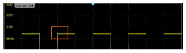
The indicated area is magnified in a new zoom diagram. The original diagram is displayed with the zoom area indicated as a rectangle.
