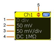
Figure 7-3: Signal label on the signal bar
