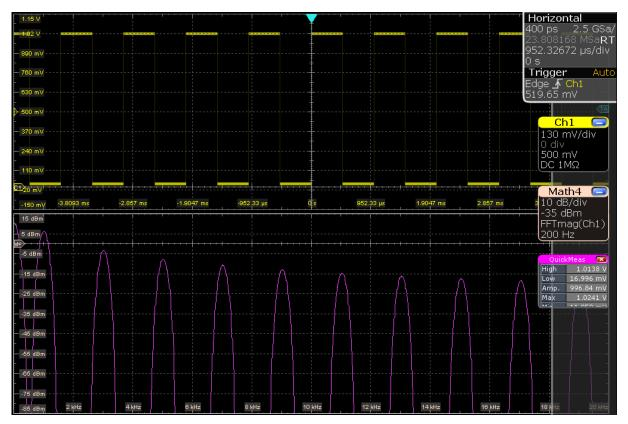
7. To remove the FFT results, tap the "Delete" icon and then the spectrum waveform.
