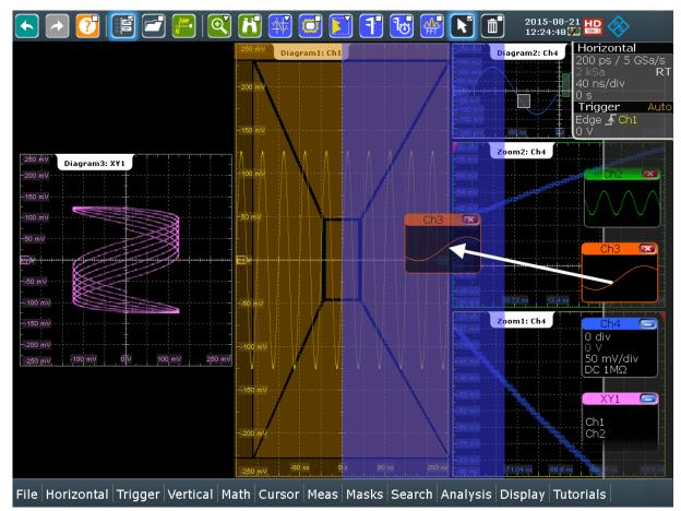
3. To change the size of the new diagram, drag its edge to the required position.
