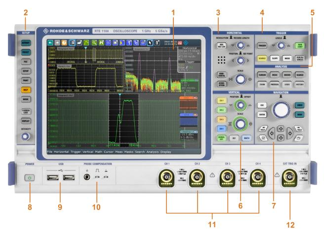
Figure 5-1: Front panel of R&S RTE1104 with 4 input channels
