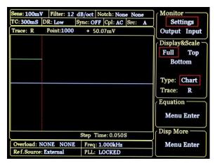
In addition, SE1022 can also uses polar coordinates to display the in-phase component and quadrature component of the input signal. All of these display modes can be easily adjusted by manual or automatic operations.
