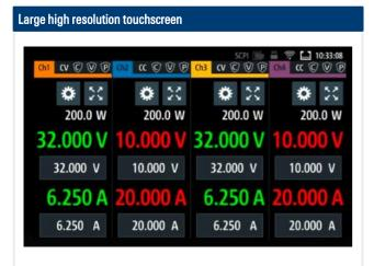
The home screen gives a clear overview of all channels. Each channel can be selected for a more detailed view containing a wide variety of additional information such as statistics and icons indicating the status of set protection levels and special functions.
