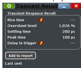
To measure and display the transient response, the instrument uses the following measurements and waveforms:
