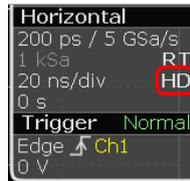
The high definition mode works with half the realtime sample rate. For FFT, the instrument halves this sample rate again.
