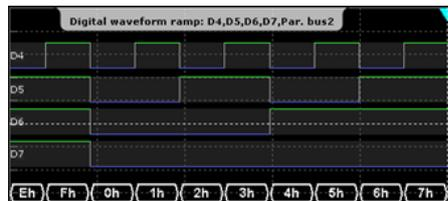
"Analog" Displays the bus values as signal amplitudes, similar to an analog waveform. Thus, a quasi-analog waveform is created.
