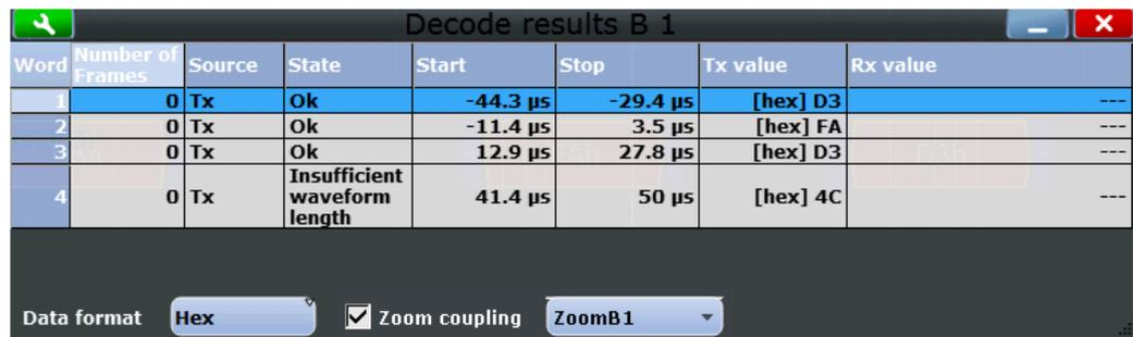
Figure 13-11: Decode results of the UART signal
