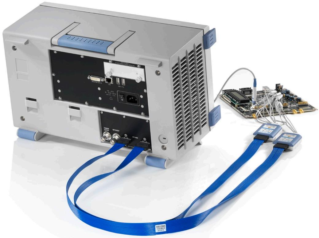
The Mixed Signal Option provides 16 digital channels grouped in two logic probes (pods) with 8 channels each. The instrument ensures that analog and digital waveforms are time-aligned and synchronized so that critical timing interactions between analog and digital signals can be displayed and tested. The automatic alignment compensates the skew between the probe connectors of the analog channels and the probe boxes of the digital channels.
