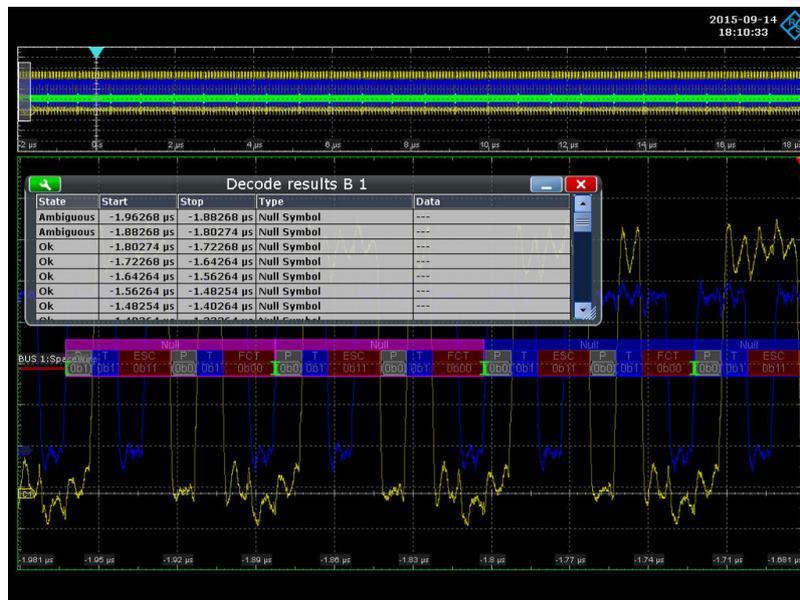
**Figure 13-111: Decoded SpaceWire signal with ambiguous bits**
