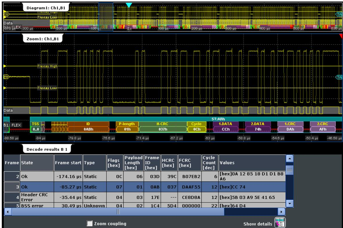
Figure 13-35: FlexRay - decoded dynamic slot and results table
