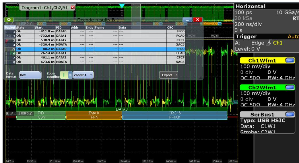
Figure 13-104: USB HSIC protocol: decoded and binary signal, and decode results
