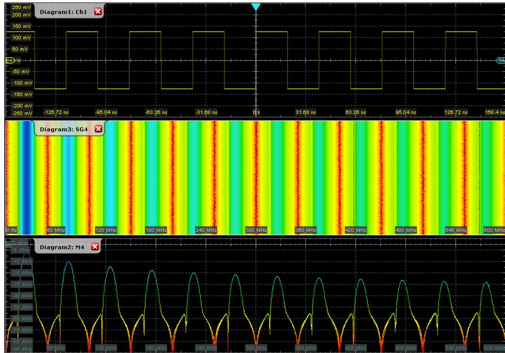
A spectrogram shows how the spectral density of a signal varies over time. The x-axis shows the frequency, the y-axis shows the time. A third dimension, the power level, is indicated by different colors. Thus you can see how the strength of the signal varies over time for different frequencies.
