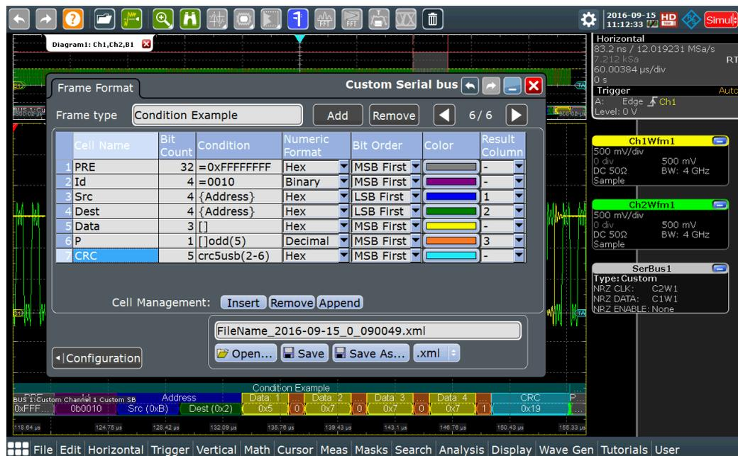
Figure 13-79: Example of a crc, parity and block frame conditions
