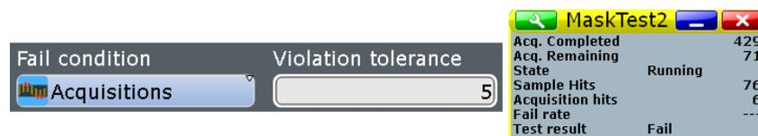
The example test has failed when the sixth acquisition violated the mask.
