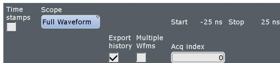
To save one waveform from the history, enter the number of the required acquisition in "Acq index", and tap "Save".
