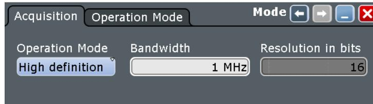
Figure 5-7: Setting the instrument into high definition mode
